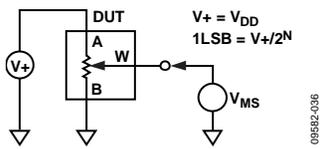
Figure 36. Potentiometer Divider Nonlinearity Error (INL, DNL)
