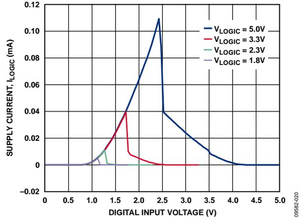
Figure 20. Supply Current ( $I_{LOGIC}$ ) vs. Digital Input Voltage
