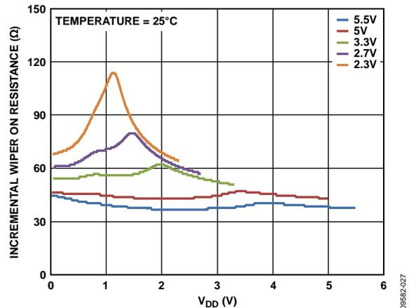
Figure 27. Incremental Wiper On Resistance vs.  $V_{DD}$
