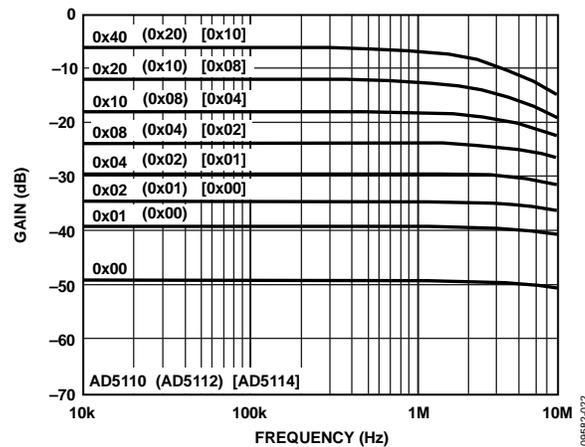
Figure 22. 10 kΩ Gain vs. Frequency vs. Code
