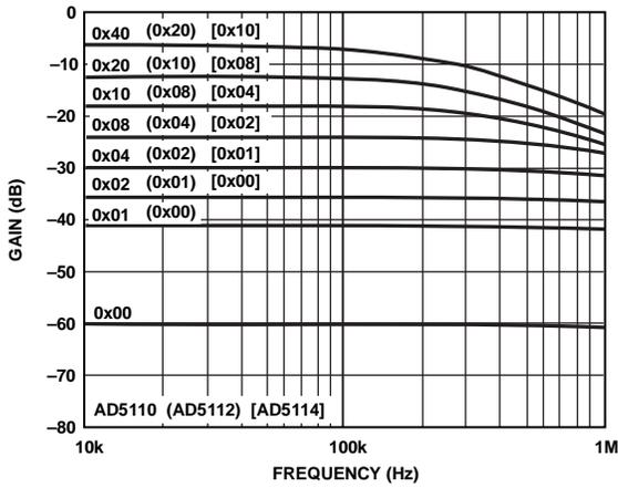
Figure 23. 80 kΩ Gain vs. Frequency vs. Code
