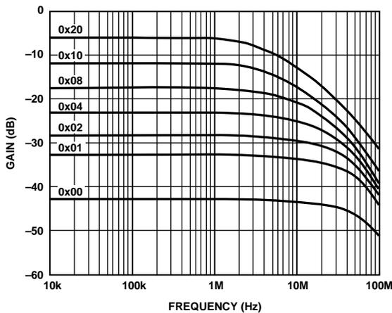
Figure 19. 5 kΩ Gain vs. Frequency vs. Code
